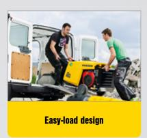
The compressor can be manually lifted via four ergonomically designed hand grips to enable easy loading into a van, for example – additional lifting gear is not necessary.
