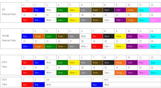
The above chart is a quick reference guide for indentification of fibers and tubes in the most common cable designs. For detailed information about the color code systems, please contact Hexatronic.
